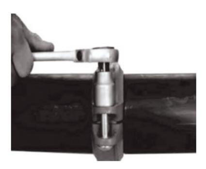
7 a. Assembly completed- Rigid Coupling
